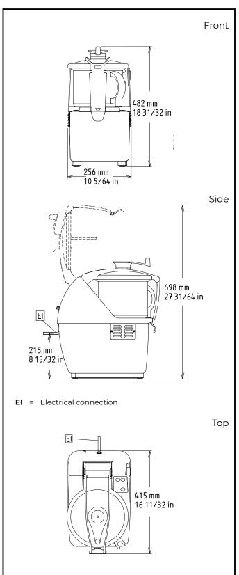
Electric **Supply voltage:** 110-120 V/1N ph/60 Hz
